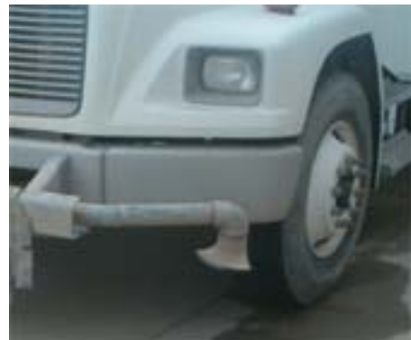
Tankers equipped with flushing nozzles are used to clean silt from pavement
