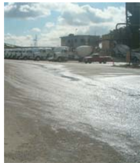
Water tracked from the wash can dry and leave fine silt behind that becomes airborne
